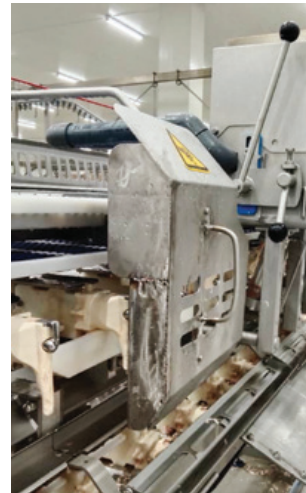
Install Machine Guarding
