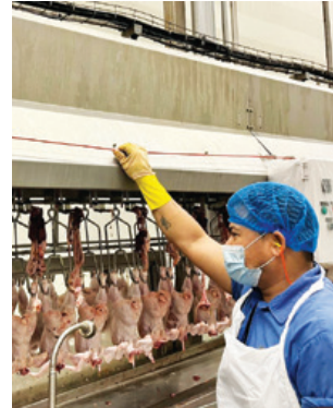
Safety Pull Cords at High-risk areas
