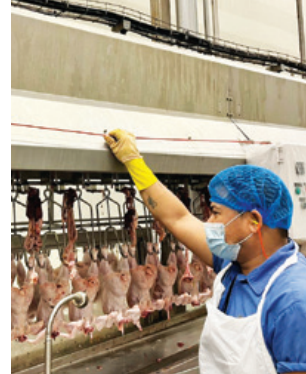
Safety Pull Cords at High-risk areas
